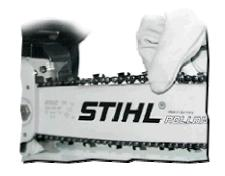
4. A correctly tensioned cold chain
